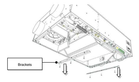
**Stage 5:** Remove the two Heat Exchanger fixing Brackets and Heat Recovery Cell.
