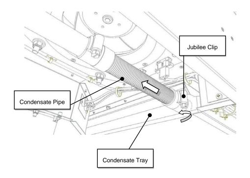
Stage 2: Loosen the Condensate Pipe Jubilee Clip and remove Pipe from Condensate Tray.
