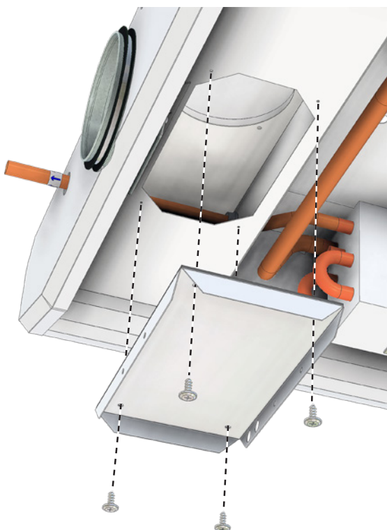
Picture 20. Opening inspection hatch.
